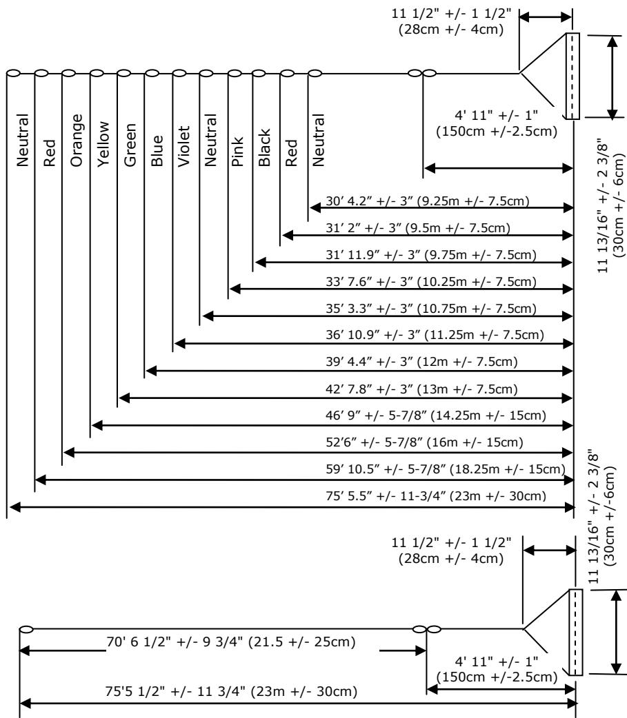
**Note:** For tournament-supplied handle sections, the bridle length shall be 150 cm  $\pm$  2.5 cm (4'11"  $\pm$  1") the triangular portion of the bridle 28 cm  $\pm$  4 cm (11 1/2 "  $\pm$  1 1/2" ), and the length of the handle 30cm  $\pm$  6 cm (11-13/16"  $\pm$  2-3/8") (see diagram). For skier-supplied handles in the Slalom and Jumping events, the tolerance on the bridal length shall be +2.5 cm/-10 cm (+1"/-4) with no tolerance on the triangular portion of the bridle.
